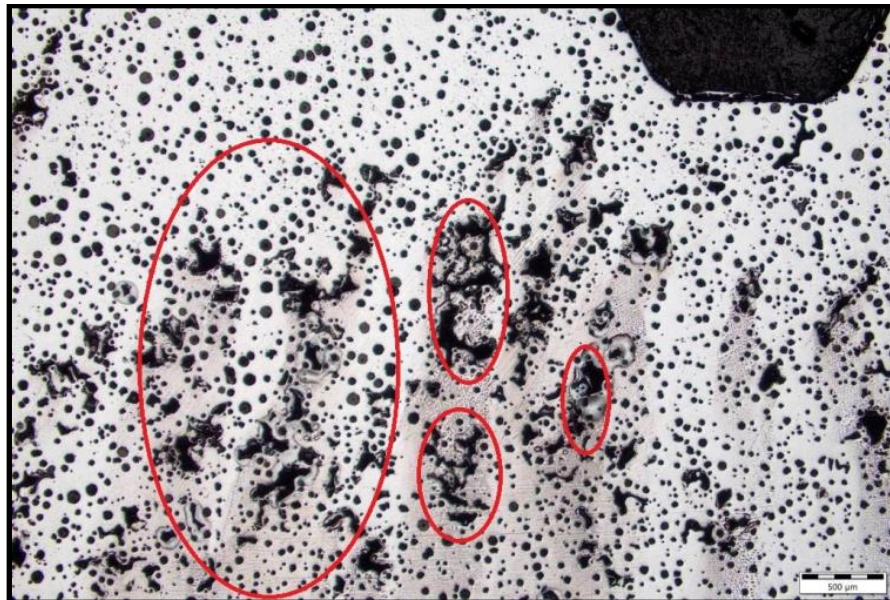
Shrinkage porosity in root of annulus gear teeth
